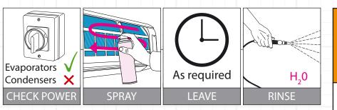
Evaporators: fan may be kept running, depending on system configuration. Condensers: turn system off.
